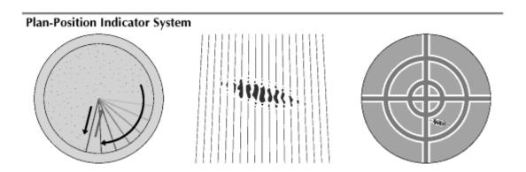
Reflected microwaves can be converted into visible images. The rotating antenna is tracked by the trace of an oscilloscope. A sweep starts at the center of the screen, left. It radiates outward at a constant rate. Reflected waves appear on the screen as a pattern of bright spots, center. On the indicator screen, right, the patterns form an image of the object' (Encyclopaedia Brittanica 2010b).
